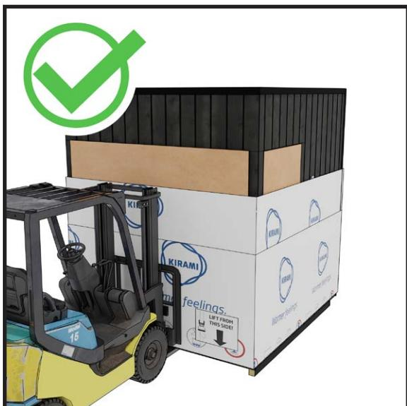
Drive forklift under the module from front.
