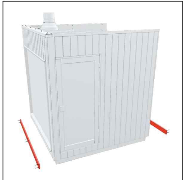
4. Make sure that there is no skirting boards attached to the modules.
