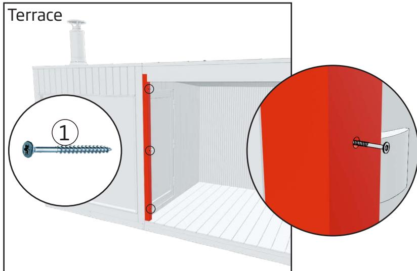
1. Attach the terrace module with three screws from the vertical post to the adjacent module.
