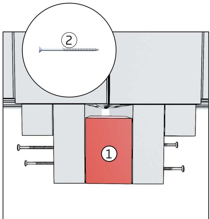
3. Attach the filler piece with four screws. Two screws from both sides.
