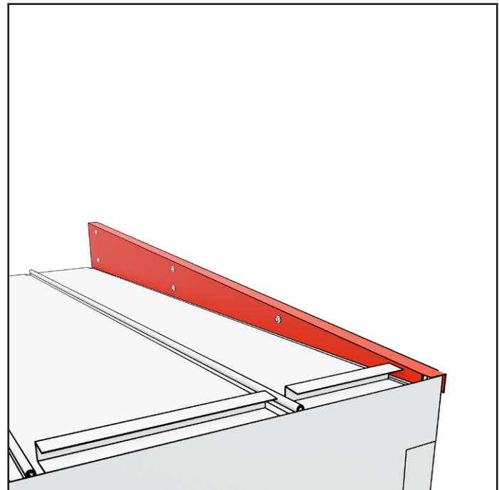
6. Attach the side flashing to the final module to be connected in the series from the same points where it was previously attached.
