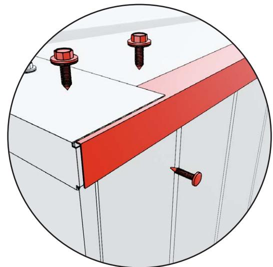
5. Make sure that the side flashings has been removed from the walls to be connected. The flashing might be tightly closed due to the presence of a silicone seam between the side flashing and the front eave flashing.
