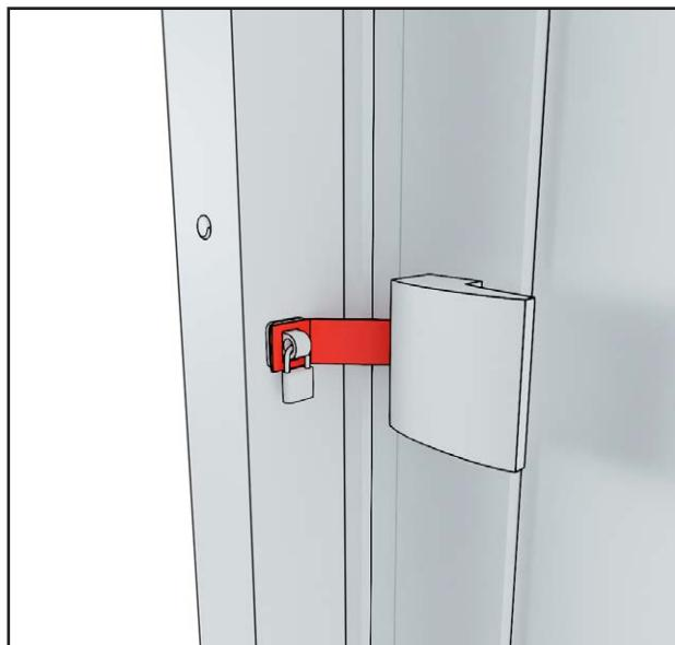
If you have installed a terrace module next to the sauna, a latch receiver must be attached to the inside of the vertical beam. This allows the sauna to be locked with a latch in accordance with regulations.
