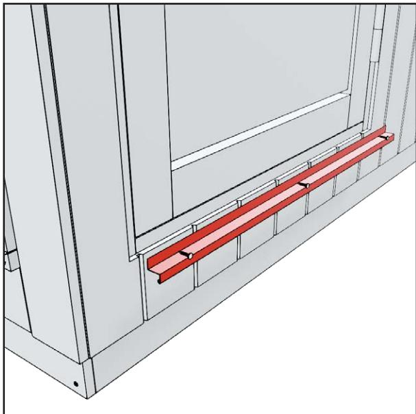
3. Make sure that there is no drip edge at the bottom of the door. Remove if necessary.
