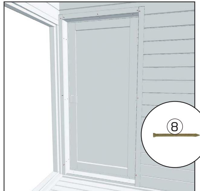
4. Finally, use cover strips to hide the gap between the cover boards and the wall.
