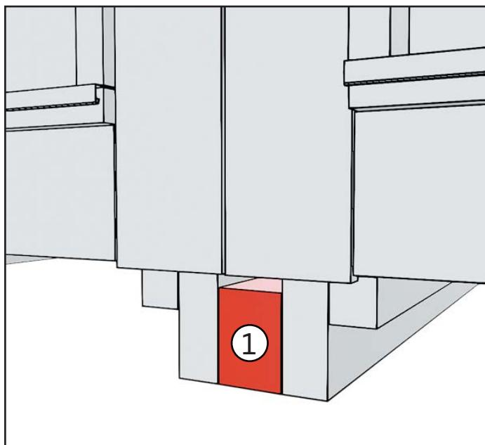
2. Place the filler piece between the transport brackets.
