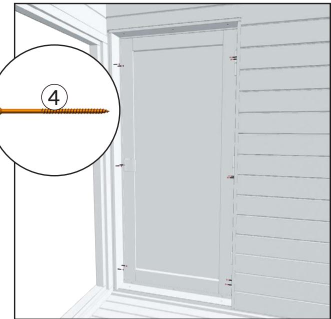
3. Fasten the long cover boards to the sides of the doorway in a way that the front edge of the boards is at the same level as the inner wall of the module.
