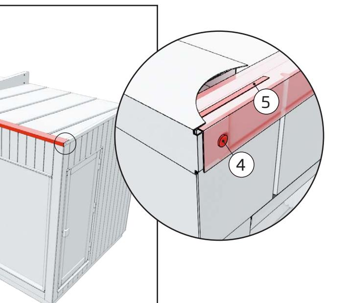
2. Place the module's eave flashing onto the roof. The eave flashing extends about 10 cm over the previous eave flashing.
