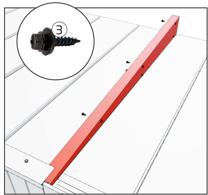
1. Place and attach the U-profile sheet between the modules. There will be five screws on both sides
