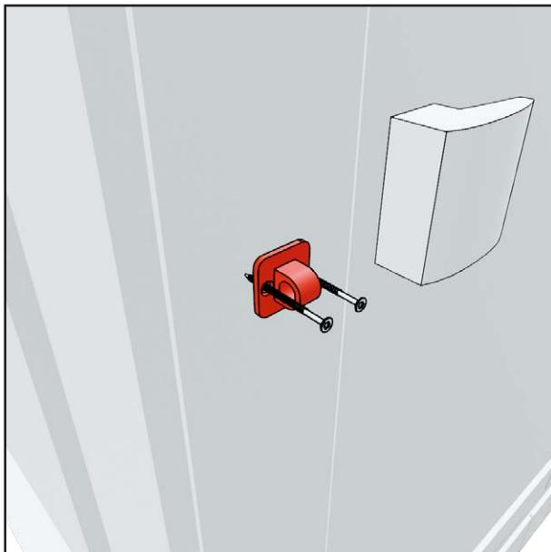
1. Make sure that the sauna door latch receiver is not attached. Remove if necessary.
