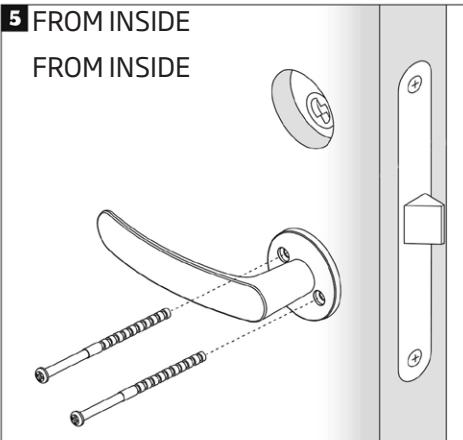
NOTE! A regular maintenance procedure is to tighten the screws of the handle after installation due to the door's shrinkage.
