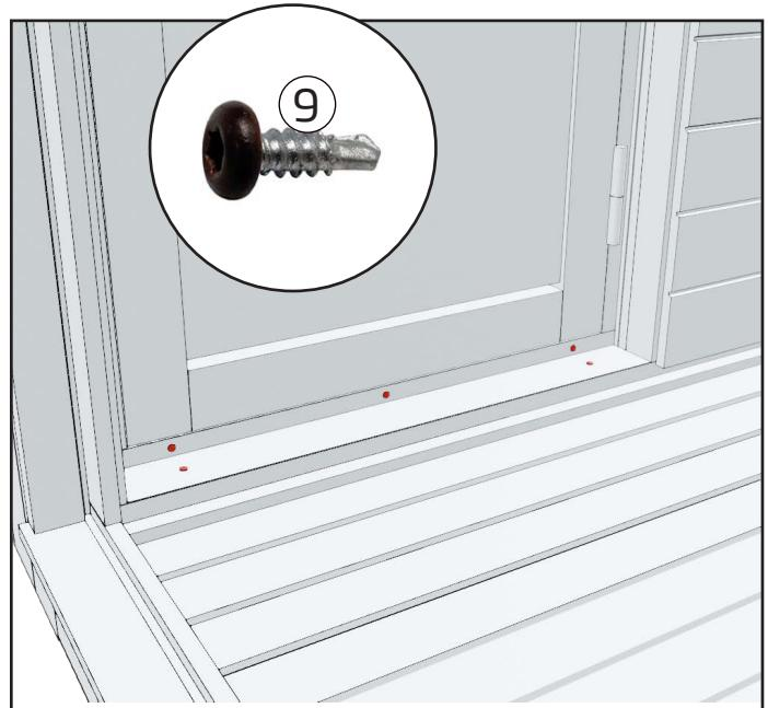
1. Place threshold plate between the modules.
