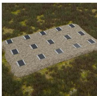
Under the modules, we recommend placing concrete slabs on top of the hard surface to lift it higher and putting roofing felt (bitumen roofing) on top of the slabs throughout the width of the slab.
