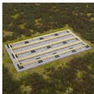
After this, it is good to make a grid (durable material) on top of the concrete slabs (Picture below) which makes it easier to get the modules on the same level.
